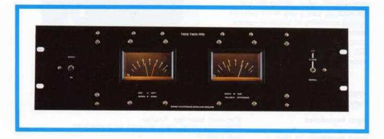
The TWIN TWIN PPM is an attractive rack mounting unit comprising two TWIN movements and two PPM9 boards to give simultaneous monitoring of A/B on Red and Green and M/S on White and Yellow pointers. Together these provide complete information about stereo signals, in contrast to the ambiguous readings of phase meters. Audio sockets provided for each channel are XLR 3 pole male and female in parallel and a 2.5 metre connector lead to BS6500 is supplied for the mains input.
