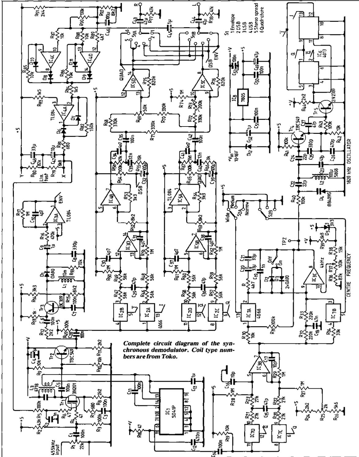
IC<sub>7C</sub> D and IC<sub>3B</sub>. A preset, R<sub>25</sub>, allows offsets to be cancelled so that the re-generated carrier is accurately in phase.
